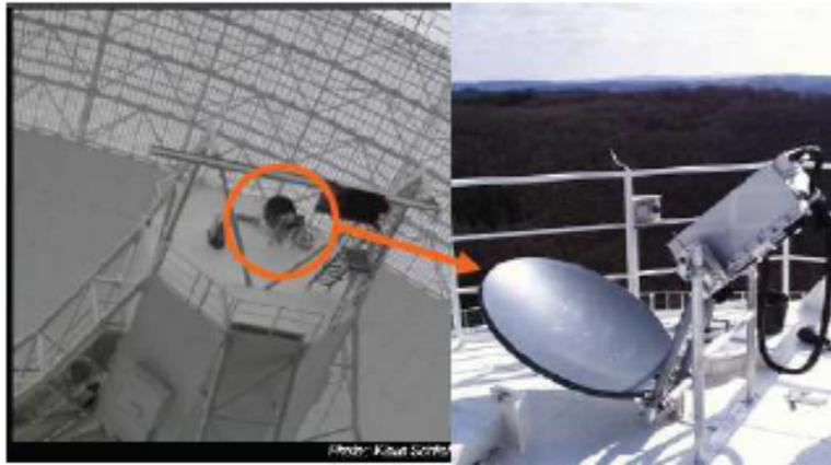
Water Vapor Radiometer
