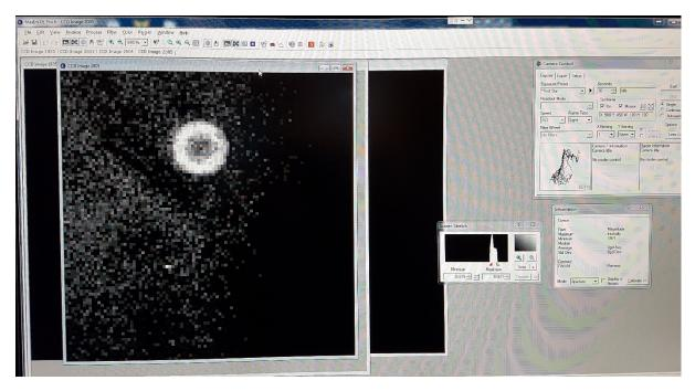
This 'donut' is the image of the output fibre. The darker area is the core of the fibre which is the location to place the image of the star. The fibre image can be placed anywhere in the camera field of view by using the two adjustments on the mirror. In operation you will see a camera image that looks like Figure 5. The spot on the left is the image of the star and the spot on the right is the reflection from the face of the output optical fibre.
